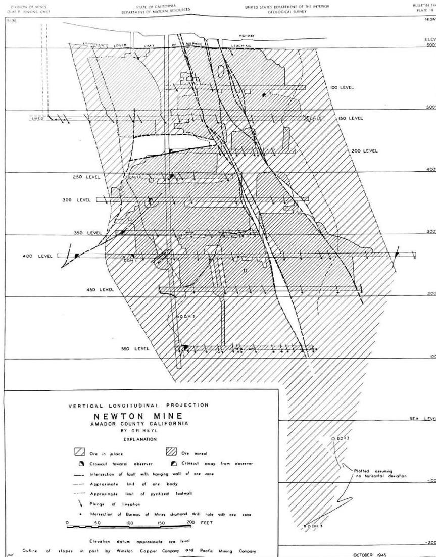
Figure 9 - Cross-section of ore body and mining levels at the Newton Copper Mine as of 1948. (Modified from Plate 10, Heyl and Eric, 1948).
